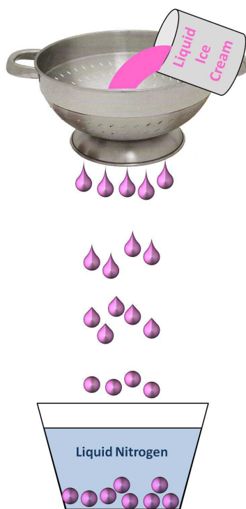
Figure 3: General method of flash freezing ice cream spheres.
